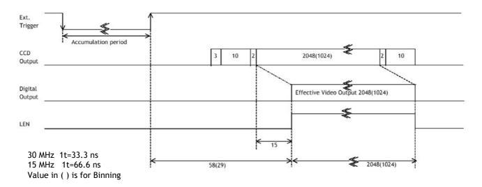
Fig. 15. Timing for external trigger shutter mode
